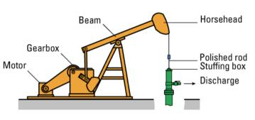
pushed) allowing oil to flow though the valve. The motor speed and torque is controlled for efficiency and minimal wear with a Pump off Controller (PoC). Use is limited to shallow reservoirs down to a few hundred meters, and flows up to about 40 liters (10 gal) per stroke.
