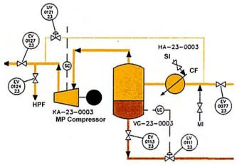
passes through the **scrubber** to remove liquids and goes into the compressor. The **anti surge** loop (thin orange line) and the surge valve (UV0121 23) allow the gas to recirculate. The components are described below.
