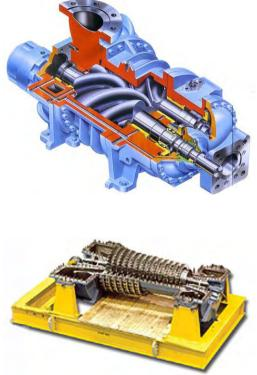
Applications include air compressors and cooling compression in LNG plants. *Axial rotor photo: Dresser Rand*
