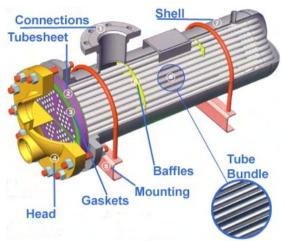
When designing the process, it is important to plan the thermal energy balance. Heat should be conserved e.g. by using the cooling fluid from the gas train to reheat oil in the oil train. Excess heat is dispersed e.g. by seawater cooling. However hot seawater is extremely corrosive, so materials with high resistance to corrosion, such as titanium must be used. *Photo: SEC Shell and Tube Heat Exchanges*
