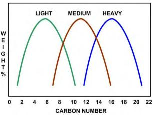
barrels of a naturally occurring 40 degree API South Louisiana Sweet crude fed to the distillation column at the refinery, could come out of the still as 1.4 barrels of gasoline and naphtha (typically  $C_8H_{18}$ ), 0.6 barrels of kerosene (jet fuel  $C_{12-15}$ ), 0.7 barrels of diesel fuel (average  $C_{12}H_{26}$ ), 0.5 barrels of heavy distillate ( $C_{20-70}$ ), 0.3 barrels of lubricating stock, and 0.5 barrels of residue (bitumen, mainly poly-cyclic aromatics).
