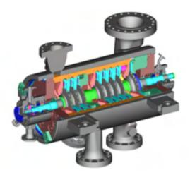
Most compressors will not cover the full pressure range efficiently. The lowest pressure is atmospheric, for gas to pipeline, some 3 to 5 MPa (30-50 bar) pressure is used, while reservoir reinjection of gas will typically require 20 MPa (200 bar) and upwards since there is no liquid in the tubing and the full reservoir pressure must be overcome. Therefore compression is divided into several stages to improve maintenance and availability.
