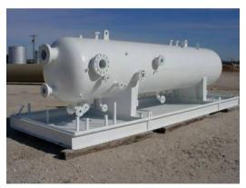
In gravity separation, the well flow is fed into a horizontal vessel. The retention period is typically 5 minutes, allowing the gas to bubble out, water to settle at the bottom and oil to be taken out in the middle. The pressure is often reduced in several stages (high pressure separator, low pressure separator etc.) to allow controlled separation of volatile components. A sudden pressure reduction might allow flash vaporization leading to instability and safety hazards.
