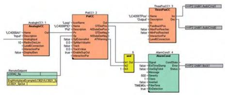
The main function of the control system is to make sure the production, processing and utility systems operate efficiently within design constraints and alarm limits. The control system is typically specified in programs as a combination of logic and control function blocks such as AND, ADD, PID. For a particular system, a library of standard solutions such as Level Control
