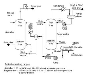
A typical amine gas treating process (as shown in the flow diagram) consists of an absorber unit, a regenerator unit and accessory equipment. In the absorber, a "lean" amine solution absorbs H2S and CO2 from the upflowing sour gas to produce a sweetened gas stream as a product. The "rich" amine solution contains the absorbed acid gases and is routed into the regenerator (a stripper with a reboiler). The stripped overhead gas from the regenerator is concentrated  $H_2S$  and  $CO_2$ .
