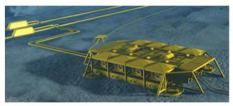
transported by undersea pipeline and riser to a processing facility. This allows one strategically placed production platform to service many wells over a reasonably large area. Subsea systems are typically in use at depths of 500 meters or more, and do not have the ability to drill, only to extract and transport. Drilling and completion is performed from a surface rig. Horizontal offsets of up to 250 kilometers/150 miles are currently possible. *Photo: StatoilHydro*
