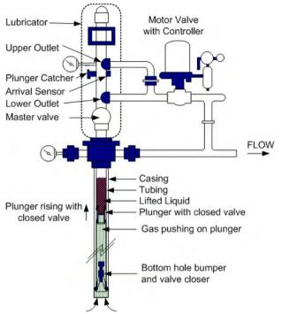
valve opens and allows gas to flow freely for some time while new liquid collects at the bottom. After a preset time the catcher will release the plunger and the cycle repeats.
