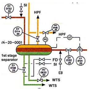
to process disturbances. LL and HH are alarm conditions and detect that the process is operating out of range and there is a chance of undesirable events and malfunction.
