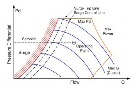
The operating characteristics are defined by the manufacturer. In the above diagram the blue lines mark constant speed lines. The maximum operating limits are set by the orange line as described above. The surge domain is the area to the left of the red surge curve.
