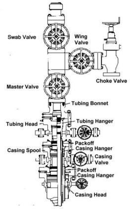
opens to the same inside diameter as the tubing so that specialized tools may be run through it. It must be capable of holding the full pressure of the well safely for all anticipated purposes. This valve is usually left fully open and is not used to control flow.
