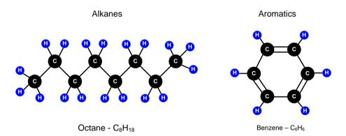
Different crude contains different combinations and concentrations of these various compounds. The API (American Petroleum Institute) gravity of a particular crude is merely a measure of its specific gravity, or density. The higher the API number expressed as degrees API, the less dense (lighter,
