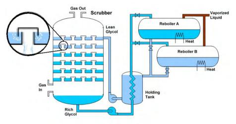
The glycol is recycled by removing the absorbed liquid. This is done in the reboiler, which is filled with rich glycol and heated to boil out the liquids at temperature of about 130-180 °C (260-350 °F) for a number of hours. Usually there is a distillation column on the gas vent to further improve separation of glycol and other hydrocarbons. For higher capacity, there are often two reboilers which alternate between heating rich glycol and draining recycled processed glycol.
