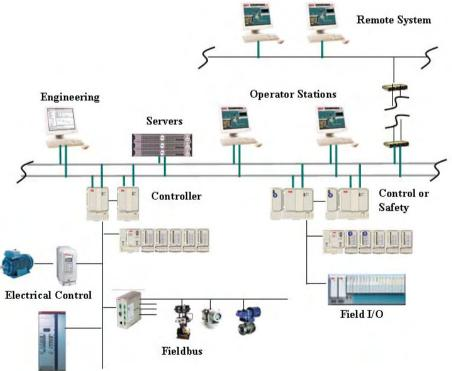
Process control systems consist of the following components:
