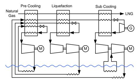
The actual design varies considerably with the different processes. The most critical component is the heat exchanger, also called the cold box, which is designed for optimum cooling efficiency. Designs may use separate cold boxes, or two stages may combine into one complex common heat exchanger.
