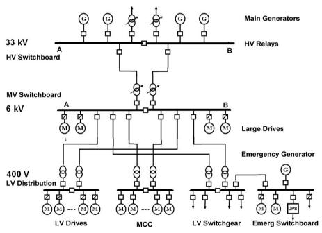
Voltage levels for high, medium and low voltage distribution boards are 13-130kV, 2-8 kV and 300-600 V respectively. Power is generated and
